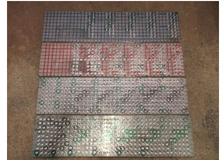
Stainless steel test plates with drilled pilot holes
