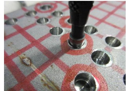
Testing of pilot hole quality
