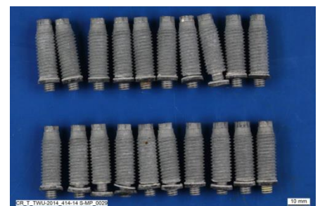
Removed S-BT HL fasteners after 12 weeks EN ISO 16701 cyclic corrosion test. No visible corrosion.
