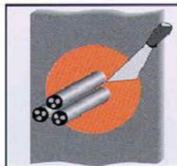
Smoothen CP 611A Sealant with a spatula
