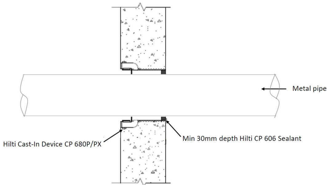
Figure 5 uninsulated metal pipes in minimum 150 mm thick rigid walls with CP 680P/PX cast-in collar.
