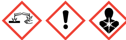
Corrosion Exclamation mark Health hazard
